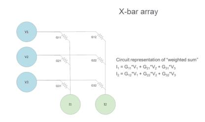
Vector Matrix Multiplication performed by sensing current; weights stored as cell conductances
