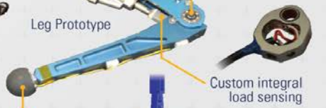
Custom contact sensor with force-sensitive resistor
