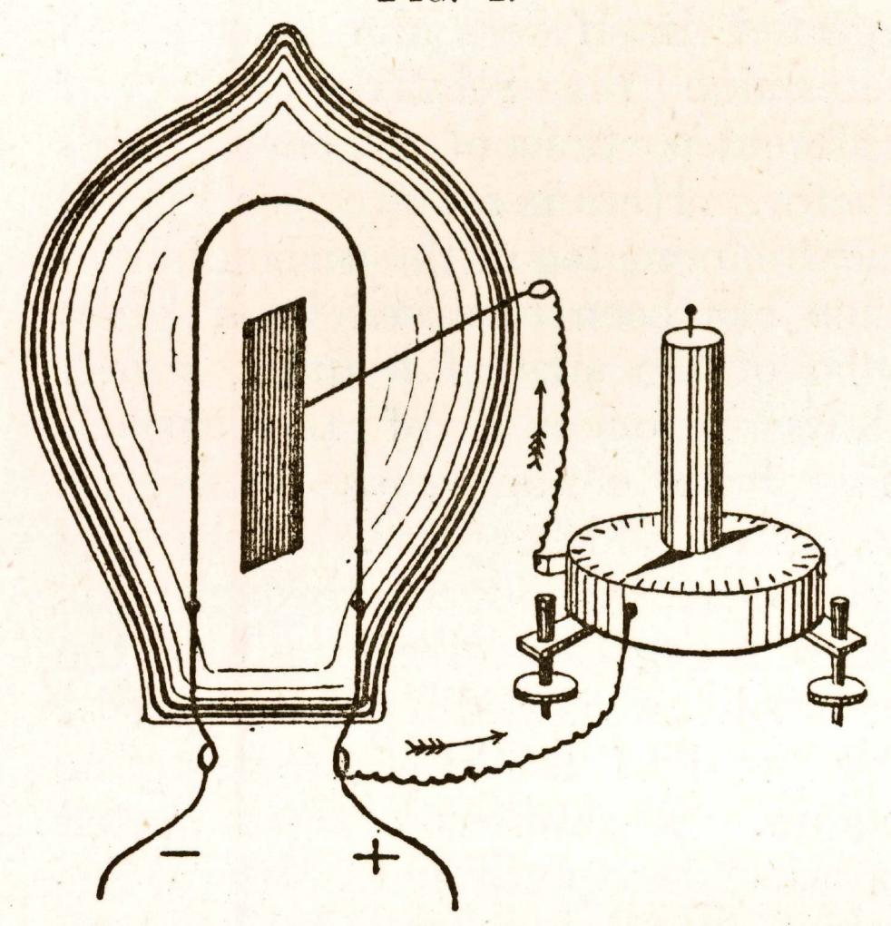
Sensitive galvanometer connected between the middle plate and positive electrode of a glow lamp, showing current flowing through it when the lamp is in action ("Edison effect").
