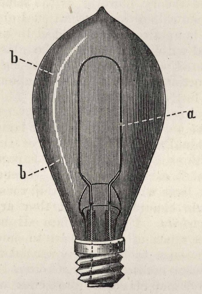
Glow lamp, having the glass bulb blackened by deposit of carbon, showing the molecular scattering which has taken place from the point a on the filament, and the shadow or line of no deposit produced at b.
