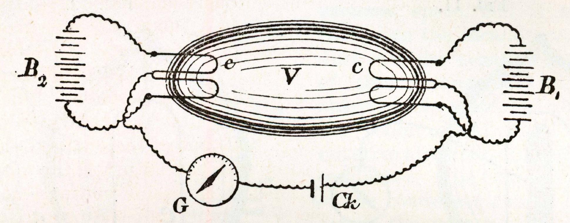
Vacuum tube having carbon loop electrodes, cc, at each end rendered incandescent by insulated batteries  $B_1$   $B_2$ , showing current from Clark cell, Ck, passing through the high vacuum when the electrodes are incandescent.
